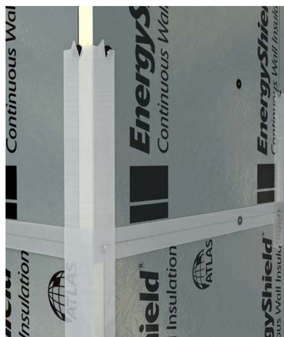
Figure 5: Apply joint sealing product at joints and all inside and outside corners, extending at least 2" on the face of board.
