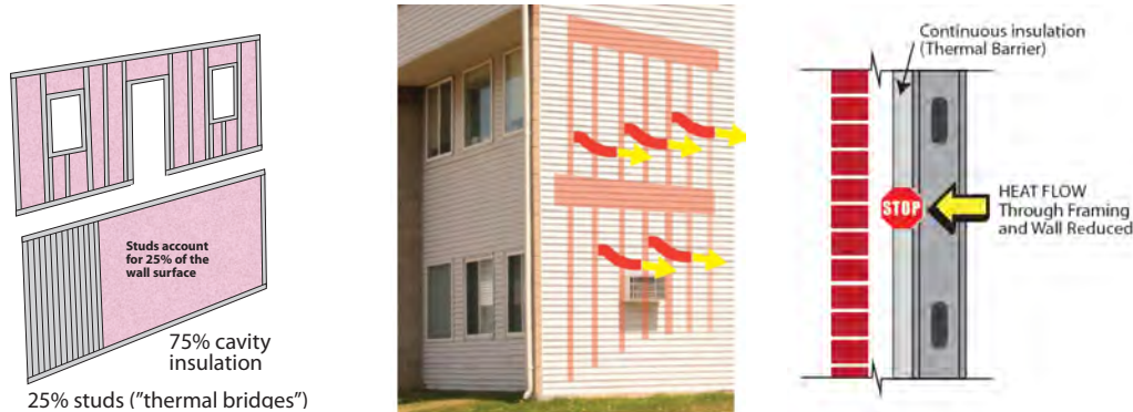
Figure 2. Thermal bridging through wall framing causes a disproportionate amount of heat loss. With continuous insulation, heat loss from thermal bridging is minimized providing a favorable economic and environmental benefit over use of cavity insulation alone.
